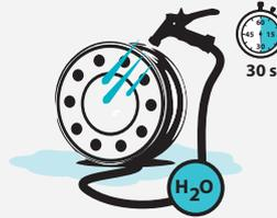
Rinse the wheel with water to prevent scratching and erosion.
