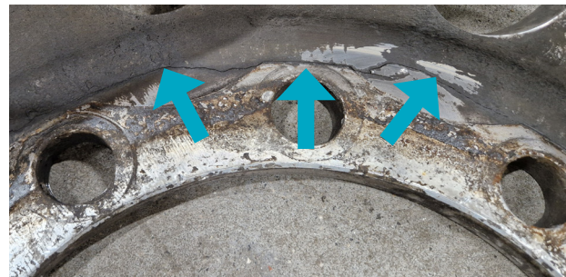
Cracks on a Non-circular hub mounted wheel
