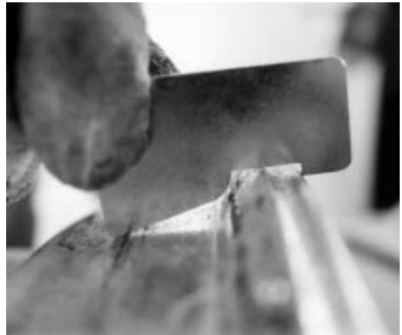
Photo 1. Acceptable Rim Flange Wear Condition
