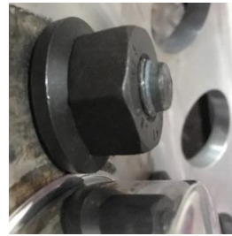
Figure 3 - Proper rear dual assembly showing inner steel wheel and outer Aluminum
