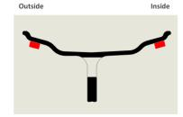
NOTE: These weights should be installed only in a location where they will not contact the brake components during vehicle operation.
