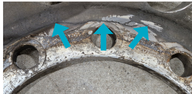
Cracks on a Non-circular hub mounted wheel
