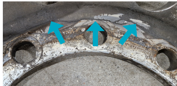
Cracks on a Non-circular hub mounted wheel
