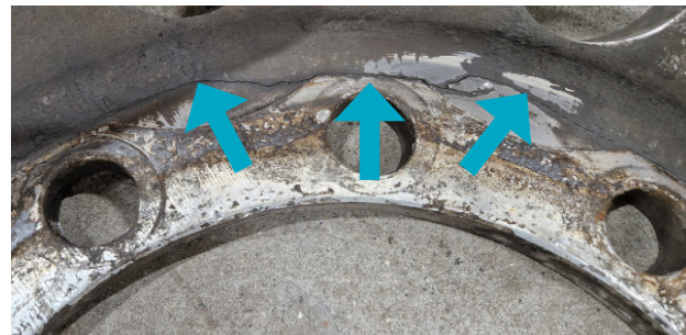
Cracks on a Non-circular hub mounted wheel
