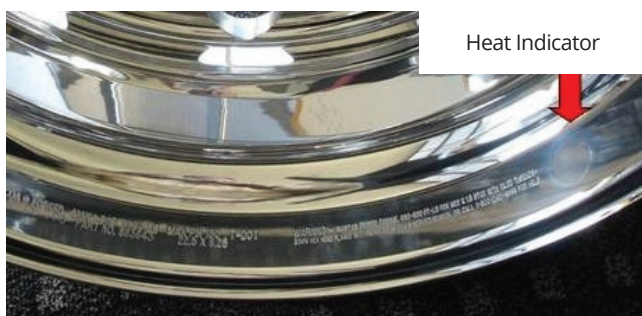
Picture 13-2 Heat Indicator at wheel flange
