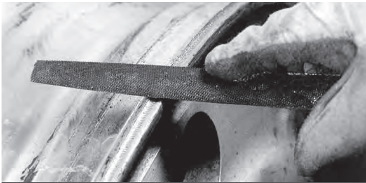
Figure 3-32: Removing sharp edge by hand with a metal file.
