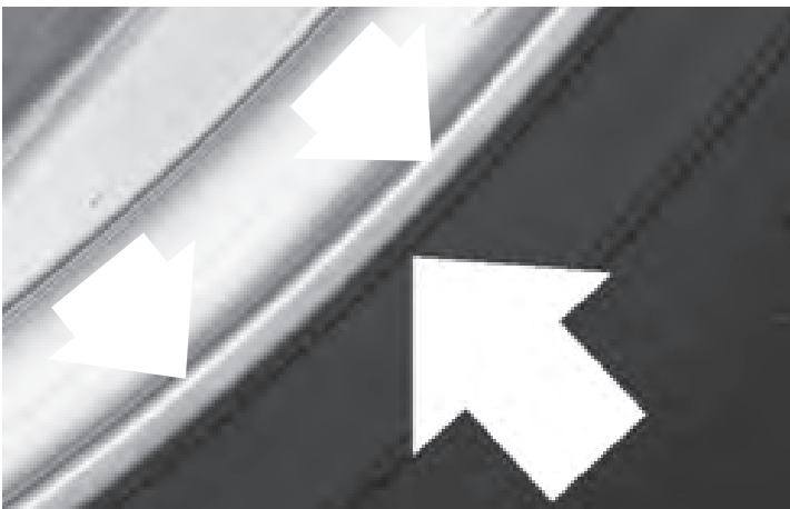
Figure 4-8: Rib evenly between arrows
