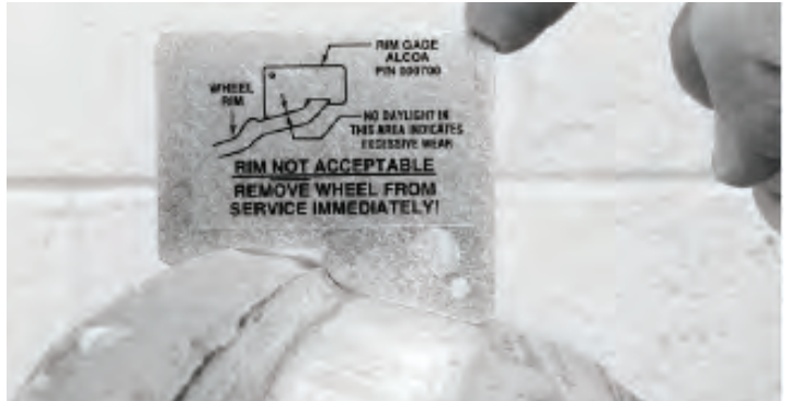
Figure 3-29: Not serviceable (scrap wheel)
