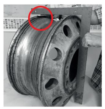
ESSA TÉCNICA DE INSPEÇÃO SE APLICA APENAS A RODAS DUPLAS OU COM FACE DE DISCO.
